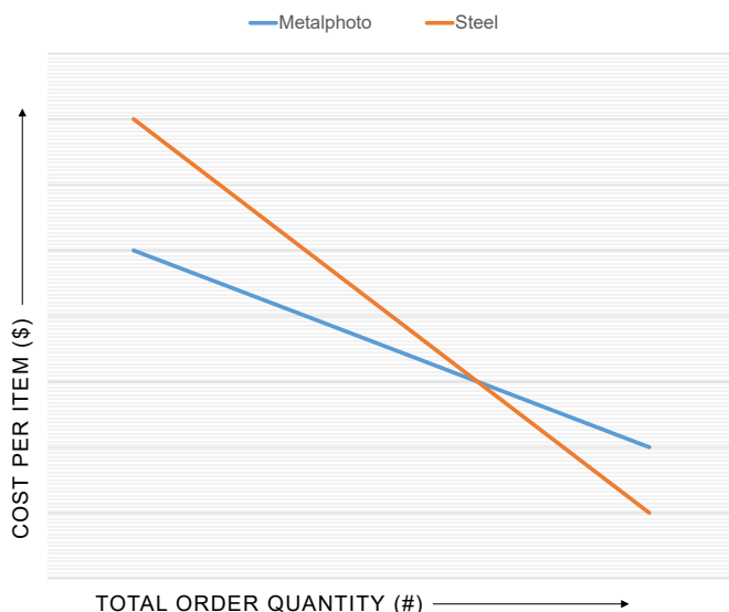
Metalphoto vs. Steel: Cost/Quantity Relationship
