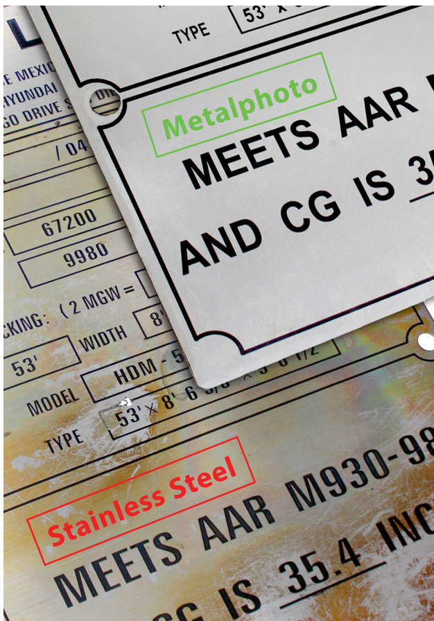
Salt spray test per ASTM B117
